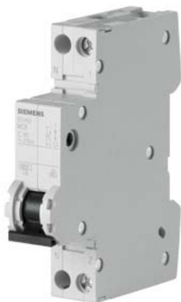
CIRCUIT-BREAKER 230 V 6 kA, 1+N-POLE/1MW, N LEFT C 40 A
