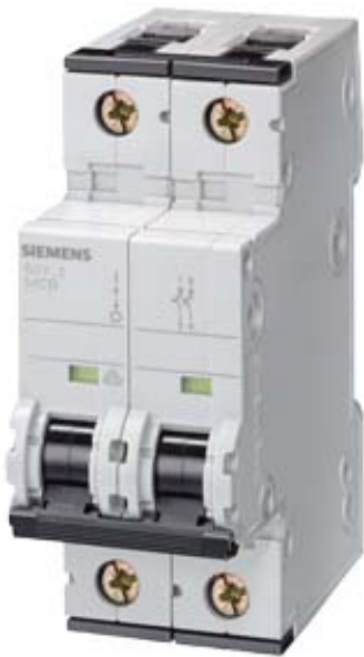
CIRCUIT BREAKER 400V 25KA, 2POLE, C, 16A, D=70MM
