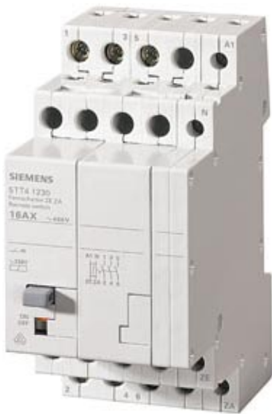
REMOTE SWITCH WITH 3 NO WITH CENTRAL ON-OFF-FUNCTION CONTACT FOR AC 230, 400V 16A CONTROL AC 230V
