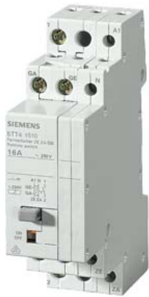
REMOTE SWITCH 1 NO CONTACT CENTRAL AND COMBINED CIRCUIT CONTACT FOR AC 230,400V 16A ACTIVATION AC 230V
