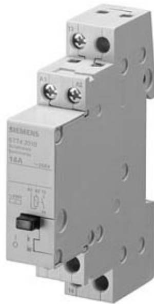
RELAY,N-TYPE W 2 CHANGE OV.CONT. CONTACT FOR AC 230V 16A CONTROL AC 24V
