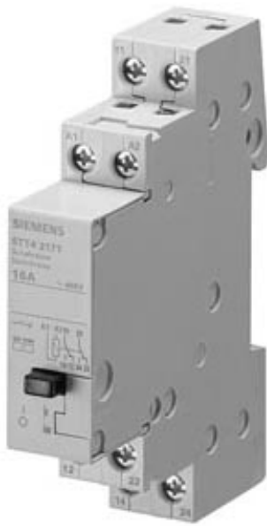
RELAY,N-TYPE W 2 CHANGE OV.CONT. CONTACT FOR AC 230, 400V 16A CONTROL DC 24V
