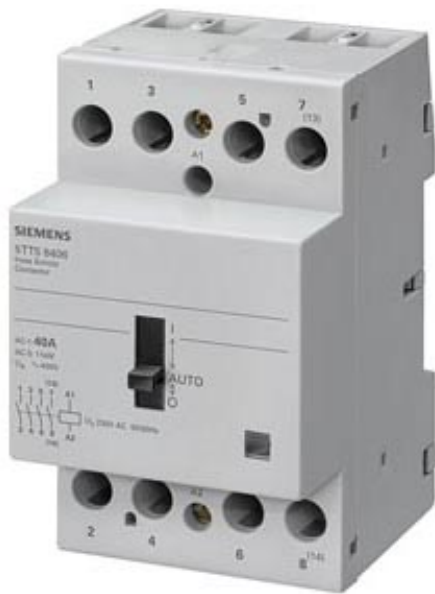
INSTA CONTACTOR 0/1 AUTOMATIC WITH 3 MAKE AND 1 BREAK CONTACT CONTACT FOR 230, 400 V AC, 40 A TRIGGERING 230 V AC
