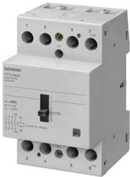
INSTA CONTACTOR 0/1 AUTOMATIC WITH 3 MAKE AND 1 BREAK CONTACT CONTACT FOR 230, 400 V AC, 40 A TRIGGERING 24 V AC
