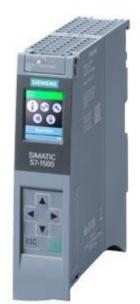
SIPLUS S7-1500 CPU 1511-1 PN T1 rail -25+55°C T1 at 70°C for 10 min with conformal coating based on 6ES7511-1AK02-0AB0 . Central processing unit with Work memory 150 KB for program and 1 MB for data, 1st interface: PROFINET IRT with 2-port switch, 60 ns bit performance, SIMATIC Memory Card required
