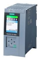
SIPLUS S7-1500 CPU 1515F-2 PN rail based on 6ES7515-2FM02-0AB0 with conformal coating, -40...+70 °C, OT4 with ST1/2 (+85 °C for 10 minutes), heat sink, no PS usable, central processing unit with work memory 750 KB for program and 3 MB for data, 1st interface: PROFINET IRT with 2-port switch, 2nd interface: PROFINET RT, 30 ns bit performance, SIMATIC Memory Card required
