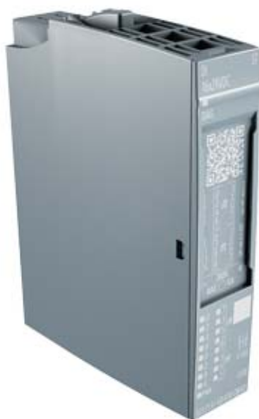
SIMATIC ET 200SP, DIGITAL INPUT MODULE, DI 16X 24VDC STANDARD, FITS TO BU-TYPE A0, COLOR CODE CC00, MODULE DIAGNOSIS
