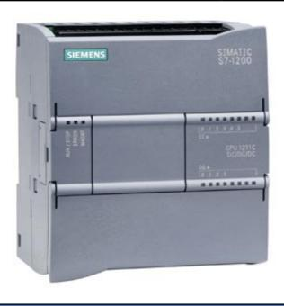
SIMATIC S7-1200, CPU 1211C, COMPACT CPU, DC/DC/DC, ONBOARD I/O: 6 DI 24V DC; 4 DO 24 V DC; 2 AI 0 - 10V DC, POWER SUPPLY: DC 20.4 - 28.8 V DC, PROGRAM/DATA MEMORY: 25 KB
