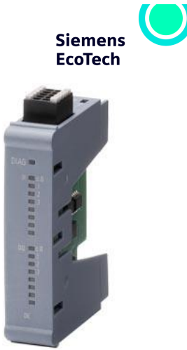
SIMATIC S7-1200 G2: SB 1231 analog input, 4 AI; inputs: 4 x AI 14 bit ADC (+/-10 V, +/-5 V, +/-2.5 V or 0-20 mA/4-20 mA)
