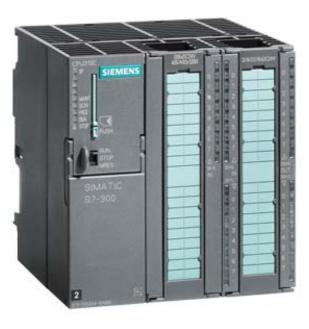
SIMATIC S7-300, CPU 313C, COMPACT CPU WITH MPI, 24 DI/16 DO, 4AI, 2AO 1 PT100, 3 FAST COUNTERS (30 KHZ), INTEGRATED 24V DC POWER SUPPLY, 128 KBYTE WORKING MEMORY, FRONT CONNECTOR (2 X 40PIN) AND MICRO MEMORY CARD REQUIRED
