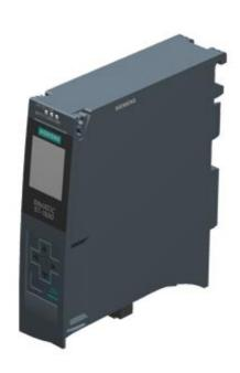
SIMATIC S7-1500, CPU 1511-1 PN, CENTRAL PROCESSING UNIT WITH WORKING MEMORY 150 KB FOR PROGRAM AND 1 MB FOR DATA, 1. INTERFACE: PROFINET IRT WITH 2 PORT SWITCH, 60 NS BIT-PERFORMANCE, SIMATIC MEMORY CARD NECESSARY
