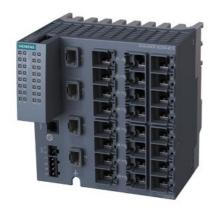
SCALANCE XC224-4C G managed Layer 2 IE switch; IEC 62443-4-2 certified; Full Gigabit; 20x 10/100/1000 Mbps RJ45 ports; 4x 1000 Mbps combo ports (either 1000 Mbps/ SFPs or 10/100/1000 Mbps RJ45 ports can be used); 1x console port; diagnostics LED; redundant power supply; temp. range -40 °C to +70 °C; mounting: DIN rail/S7 mounting rail/wall; redundancy functions; Office features (RSTP, VLAN,...); PROFINET IO device; Ethernet/IP-compliant; C-plug slot;
