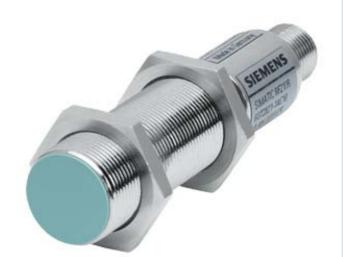
SIMATIC RF200 READER RF210R; RS422-INTERFACE (3964R); IP 67, -25 UP TO +70 DGR/C; M18 X 71 MM; WITH INTEGRATED ANTENNA.
