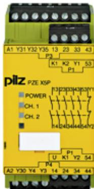
Contact expansion Inputs: 1-/2-channel wiring with/without detection of shorts across contacts Outputs: 5 N/O, 2 semiconductor. UB 24 V DC, width: 45 mm, plug-in terminals of screw type. Contact block for contact expansion in connection with safety-related control components.
