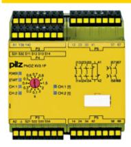
Safety relay (standalone) Inputs: 1-/2-channel wiring with/without detection of shorts across contacts Outputs: 3 N/O, 1 N/C, 2 N/O (t = 0 - 3 s). Automatic/monitored start UB 24 - 240 V AC/DC, width: 90 mm, plug-in spring-loaded terminals. Monitoring E-STOP, safety gates.
