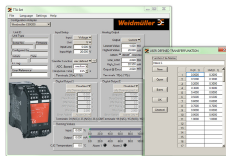
example of user defined transfer function for assigning customized output values
