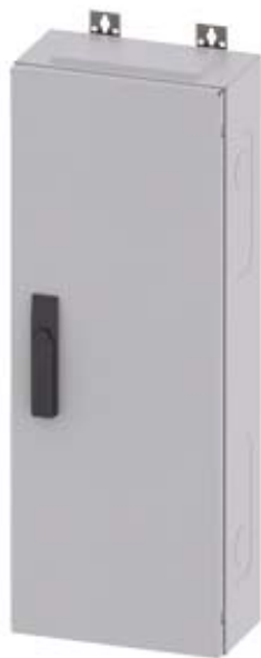
ALPHA 160 DIN, WALL-MOUNTED DB, FM UNEQ. DISTR. BOARD RAL 9016 IP31 SK2, H=800 W=300 D=140
