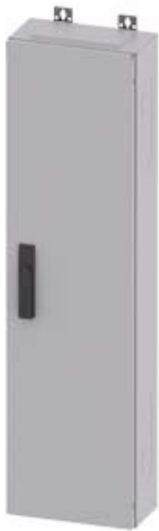
ALPHA 160 DIN, WALL-MOUNTED DB, SM UNEQ. DISTR. BOARD RAL 9016 IP43 SK2, H=1100 W=300 D=140
