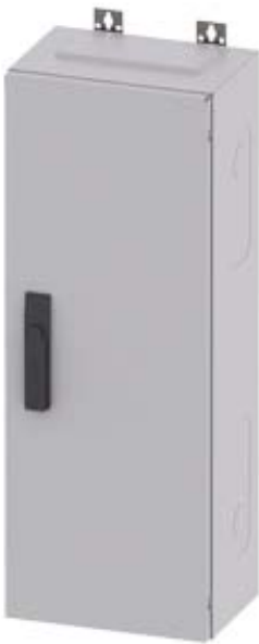
ALPHA 400 DIN, WALL-MOUNTING DISTRIBUTOR, DELIVERY FORM FLAT PACK, AP-CUBICLE, RAL 9016, IP43 SK1, H=800 W=300 D=210
