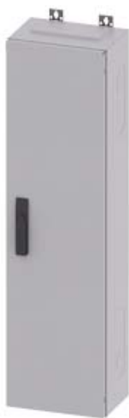
ALPHA 400 DIN, WALL-MOUNTING DISTRIBUTOR, EMPTY CUBICLE, AP-CUBICLE, RAL 9016, IP43, SK2 H=1100 W=300 D=210
