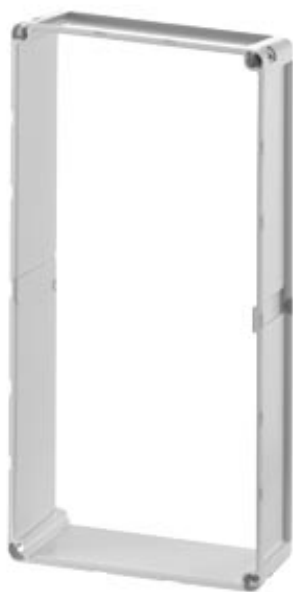
INTERMED. FRAME F. INCREASING MOUNTING DEPTH BY 92.5 MM FOR ENCLOSURE SIZE 3
