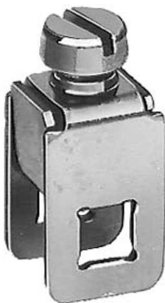
TERMINAL 1-POLE, FOR BUSBAR 6 X 6 CONDUCTOR CONNECTION 1 X 2,5- 16MM 2
