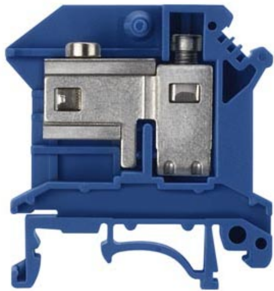
ISOLATING TERMINAL WITH SCREW CONNECTION, SECTION: 16 MM 2 WIDTH: 12 MM, COLOR: BLUE
