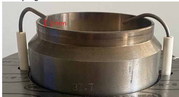
Figure 1: Spark Gap Measurement
