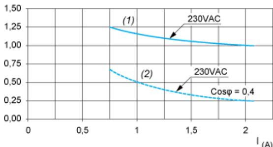
AC12 control of resistive loads and of solid state loads isolated by optocoupler,  $\cos \phi \geq 0.9$ .
