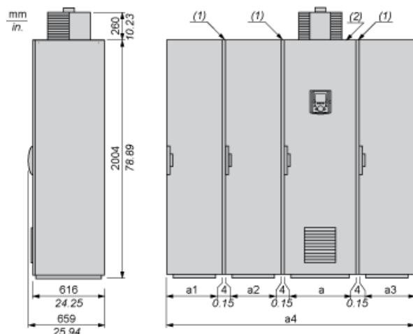
(1) Seal. For each floor-standing enclosure added, allow a 4 mm/0.15 in. space for the seal.
