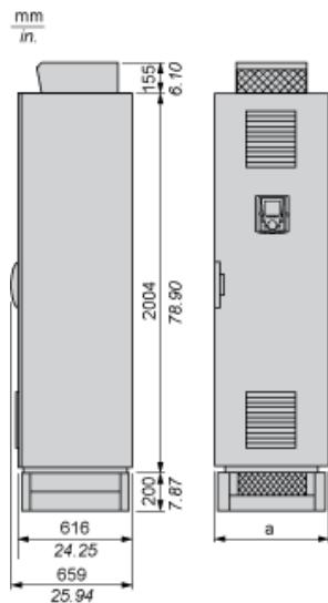
Standard Compact Floor-Standing Enclosure + Additional Floor-Standing Enclosures, According to the Configuration
