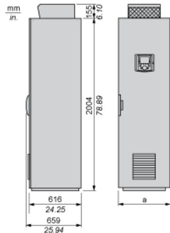
Standard Compact Floor-Standing Enclosure + Additional Floor-Standing Enclosures, According to the Configuration
