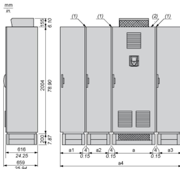
(1) Seal. For each floor-standing enclosure added, allow a 4 mm/0.15 in. space for the seal.
