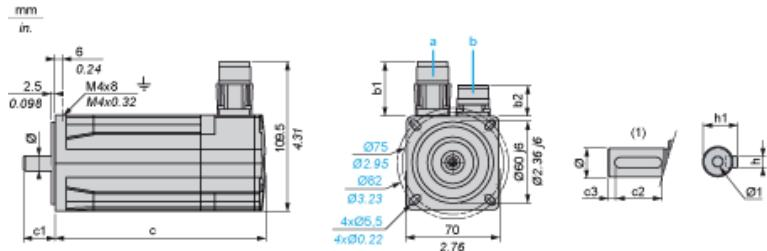
a: Power supply for servo motor brake
