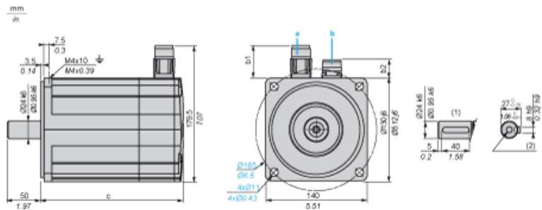
a: Power supply for servo motor brake
