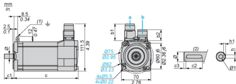
a: Power supply for servo motor brake
