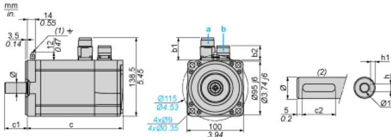
a: Power supply for servo motor brake
