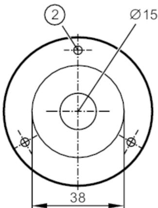
1 threaded hole M4 to fix the target on the valve piston
