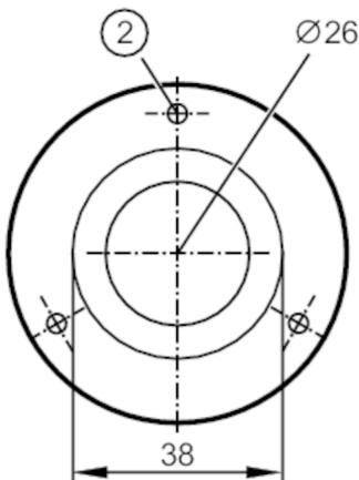
1 threaded hole M5 to fix the target on the valve piston
