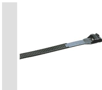
Outdoor cable ties, made in PA12, are indicated to fix devices and cables also in presence of low temperature. From sizes 9x265 mm are available ties with double heads that increase the tensile stress resistance.
