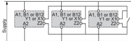
Connection of an External Control Contact Without Using Terminal Z2
