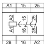
Recommended Application Wiring Diagram
