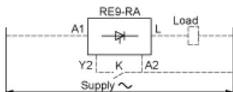
The timing relay is placed in series with the load whose de-energisation is to be delayed. Switch K is connected to terminals Y2 and A2 of the timing relay, and terminal A2 is connected to the main supply, as indicated in the diagram above. The device is operated from an a.c. mains supply whose voltage is between 24 V and 240 V.
