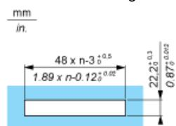
Mounting on DIN Rail with Accessory REG24PSOC
