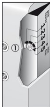
Choice of sensitivity range, dimensions in mm/m (inch)
