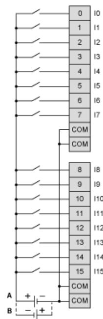
The 4 COM terminals are connected internally
