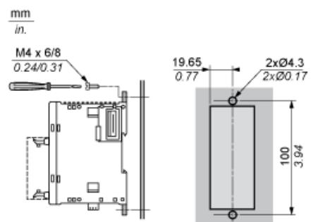
Digital Mixed I/O Module (24-channel)
