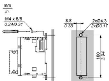
Digital Relay Output Module (8-channel)
