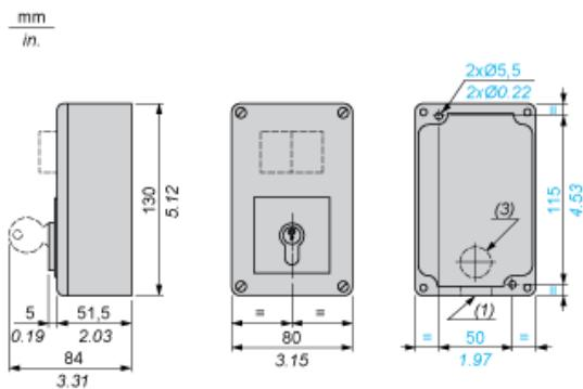
(1) 1 tapped entry for 12 mm/0.47 in. maximum capacity cable gland.
