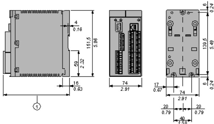
1 When using XPSMCTS• connectors this dimension is 153 mm (6.02 in)
